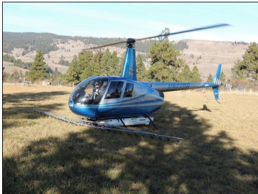
A Robinson 44 helicopter preparing to apply herbicide to a 50-acre field in the Tarpiscan Creek area
