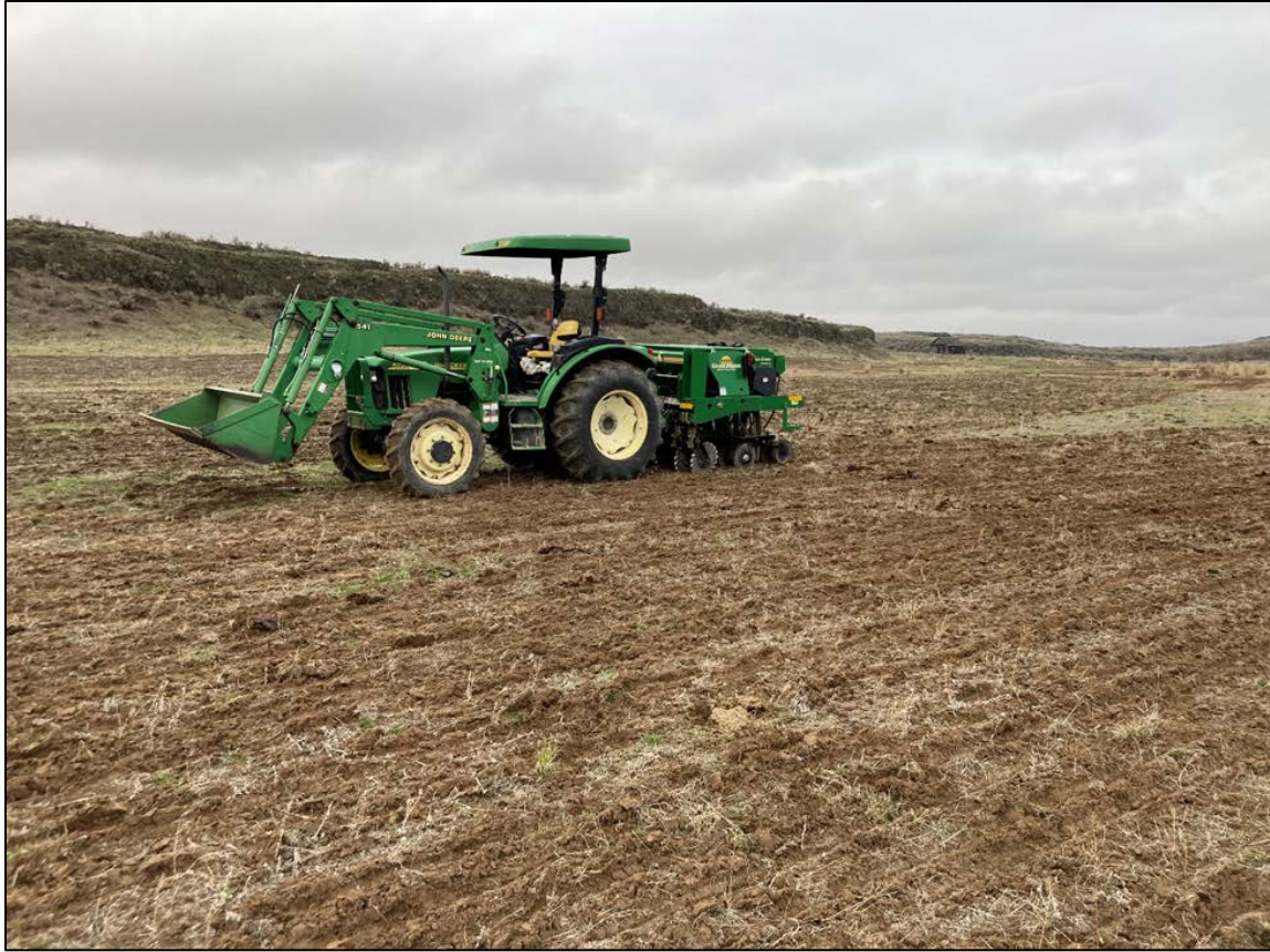
WDFW tractor and not-till drill used for seeding grasses near Lind – Photo by Nathan Cook, WDFW
