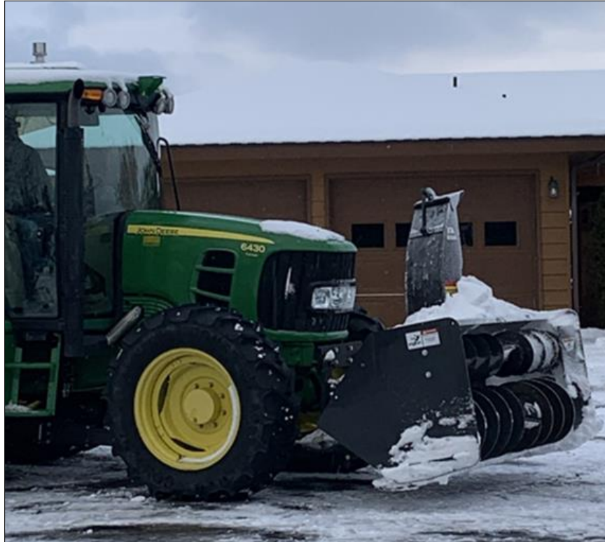
A John Deere 6430 with large snowblower on call for emergency snow removal for elk feeding in the L.T. Murray Wildlife Area
