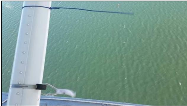
*The space between the float and the string represents the viewing window for the 50-meter survey transect*
