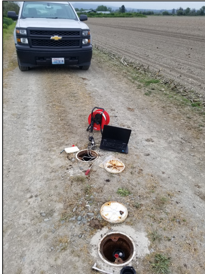
This photo shows data being uploaded onto a computer from a logger that is within a groundwater well
