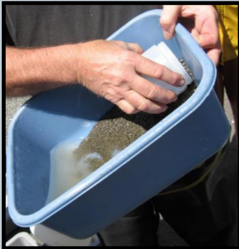
Dish pan method: Winnowing separation
