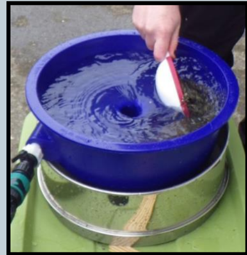
Blue bowl method: Cyclonic separation
