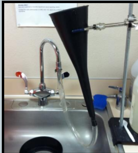
Funnel method: Elutriation separation
