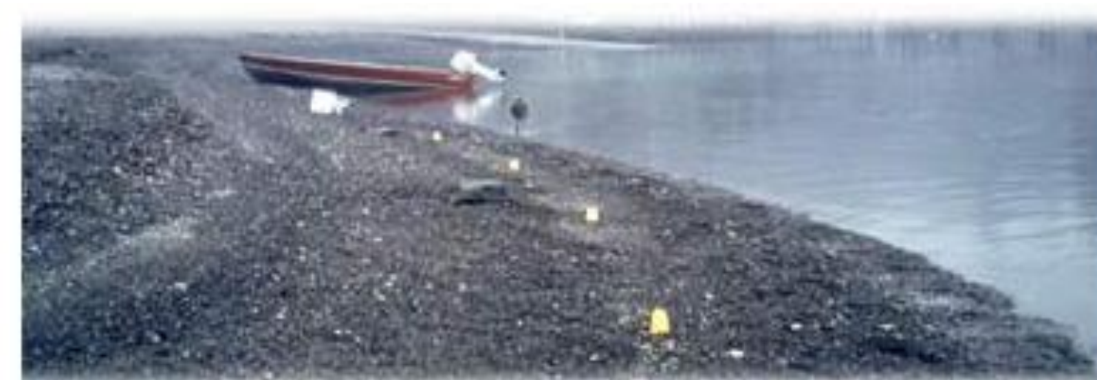
Figure 2. A sample at a site consisted of 4, 475 ml scoops of sediment taken at 6 m intervals at each of two beach elevations. This photo shows location of 4 scoop subsamples at a single beach elevation
