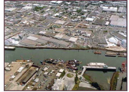
The Duwamish River. The estuary and tideflats were filled to make land more suitable for building upon and a channel was excavated for shipping. DOE photo
