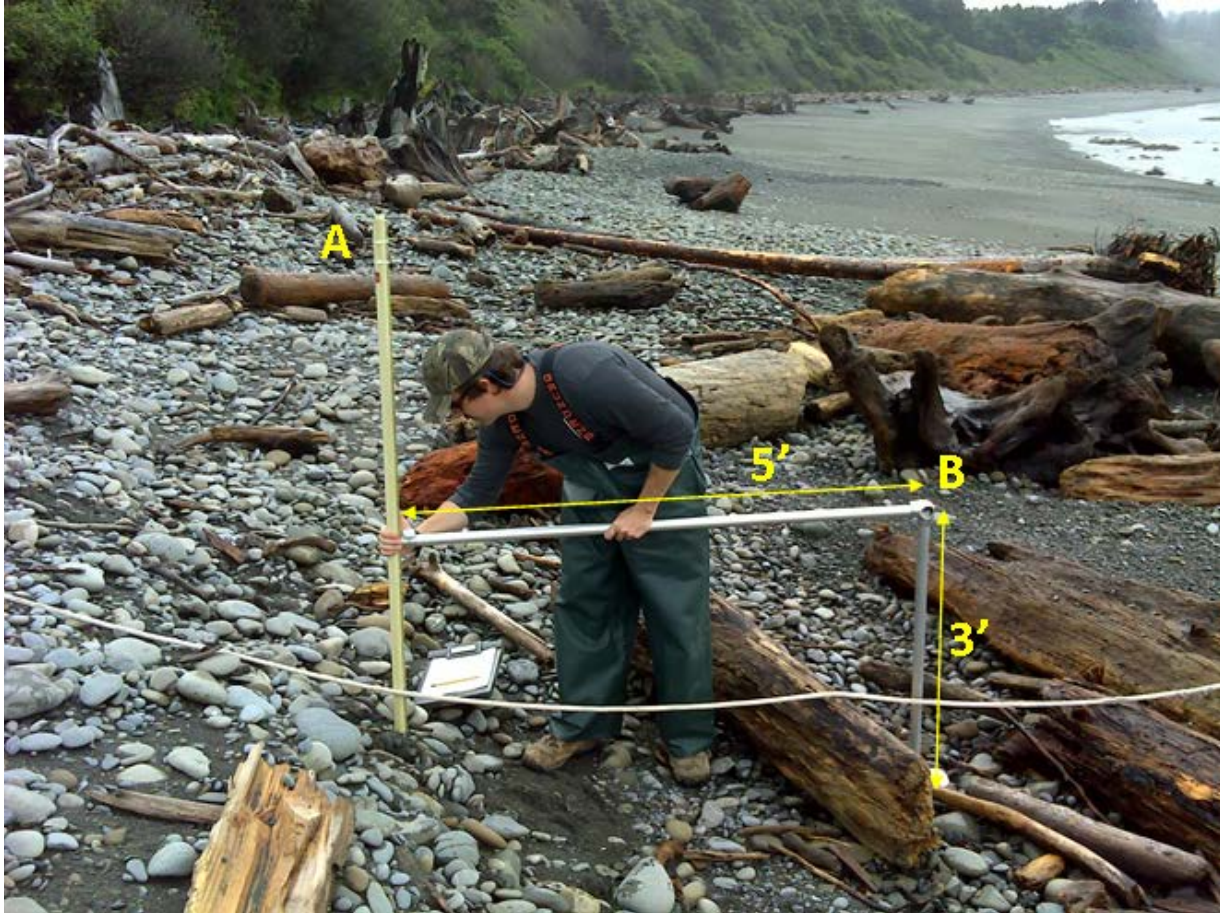
Appendix Figure 1. Beach profiling sampling apparatus: A) Stadia rod with attached level, B) Aluminum setsquare consisting of a 3 ft. vertical rod and 5 ft. horizontal rod with attached circular level.
