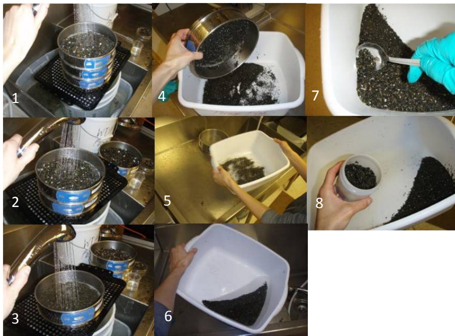
Figure 6. Sieving and winnowing process. Numbers to the lower left of each frame indicate the sequential process of sieving and washing (1-4), agitating (5), and winnowing the light fraction (6-8).
