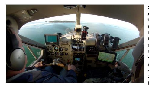
Figure 5. View of the cockpit with computing devices showing navigation and event logging software used by navigator and transect navigation software used by pilot.
