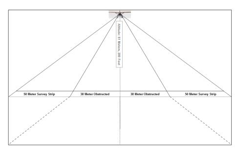
Figure 3. Diagram of left and right survey strips in relation to the transect line. An area 76 meters wide is obstructed from view directly below the aircraft due to the floats. A 50 meter transect strip is viewed from above the floats and out
