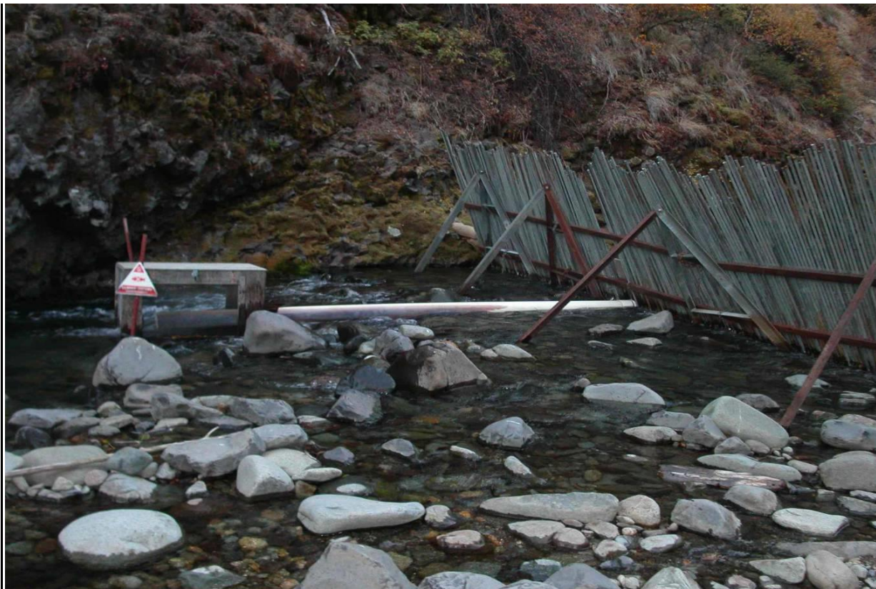
Figure 4. Rattlesnake Creek pipe weir and live box trap.
