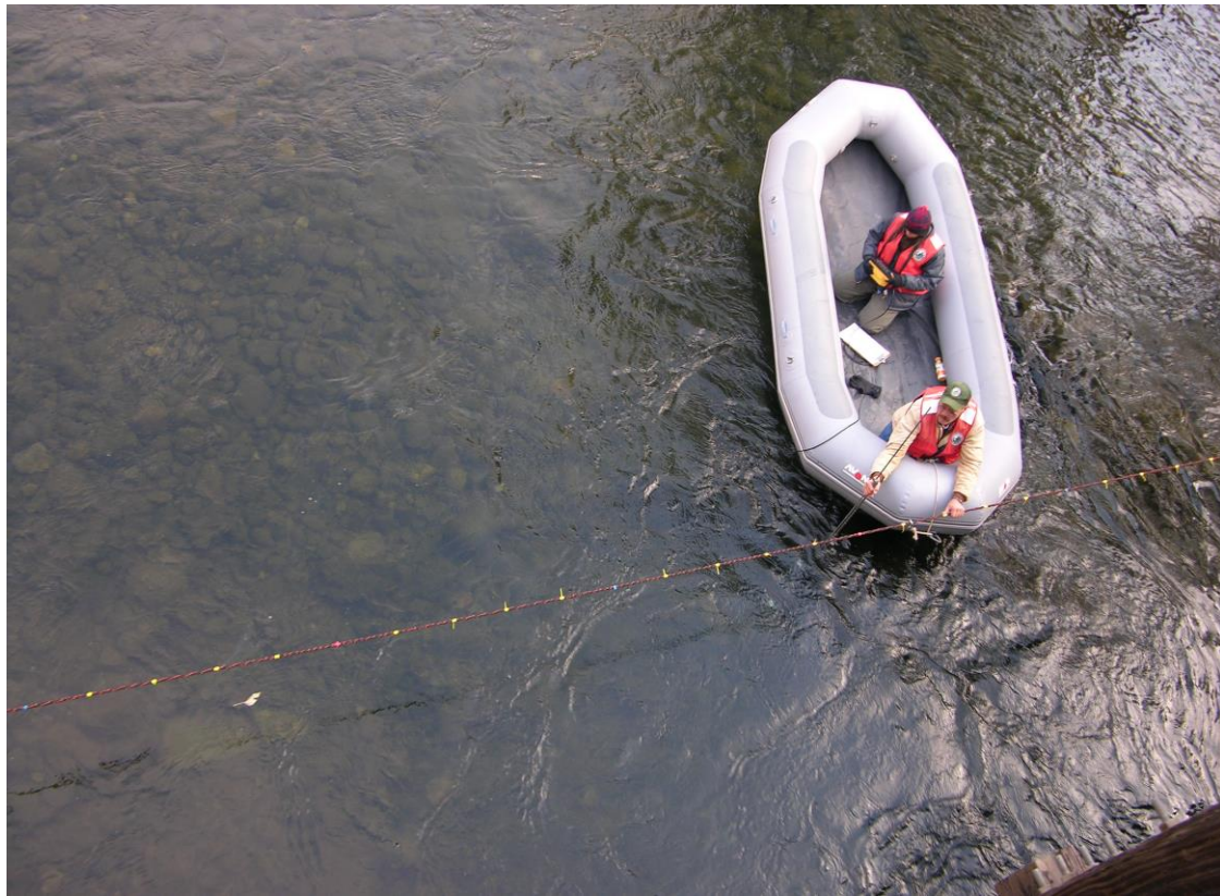
Figure 41. Naches River velocity measurements in a bull trout holding pool.
