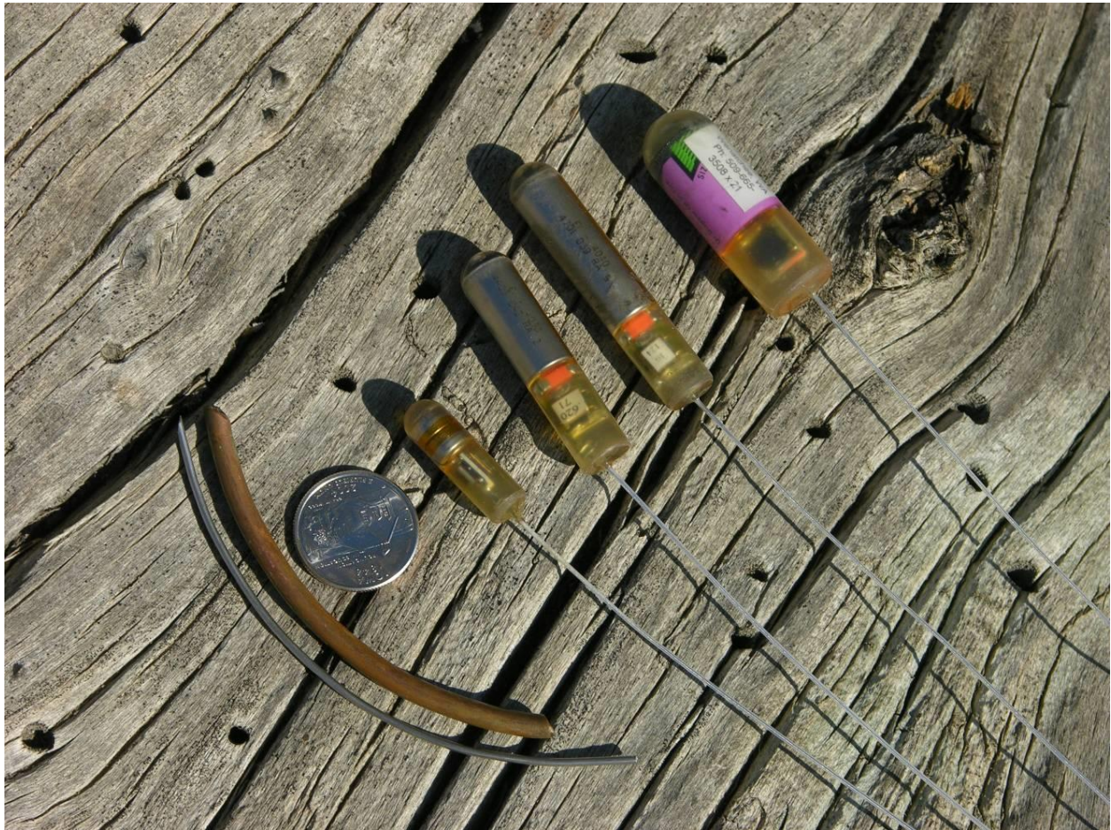
Figure 7. Four sizes of radio-tags used in bull trout surgical implants. Also shown is the steel catheter needle and copper “stinger” used in guiding the antenna lead through the fish’s body cavity.
