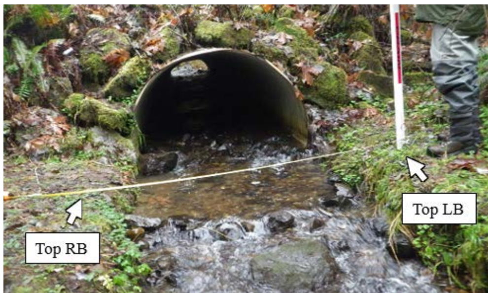
Figure 3.23. Setting up Downstream Control Cross-Section for Level B hydraulic analysis. Looking upstream toward the control and culvert, the left bank is on the right side of the photo. Secure the zero end of a measuring tape at the top of left bank (Top LB) and stretch to the top of right bank (Top RB), across the downstream control.
