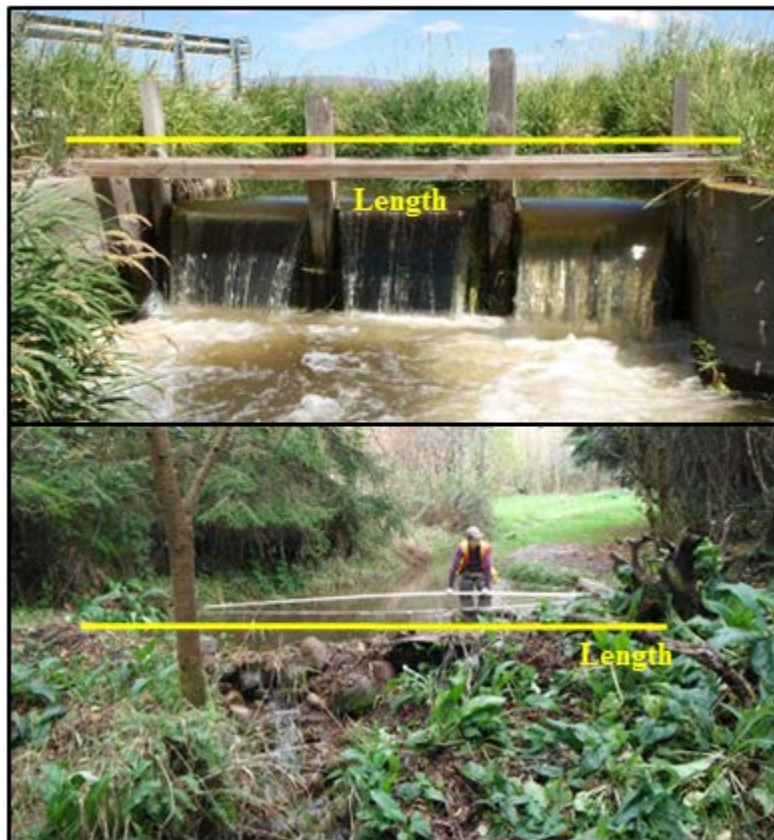
Figure 5.4. Photographic examples of dam length measurements.
