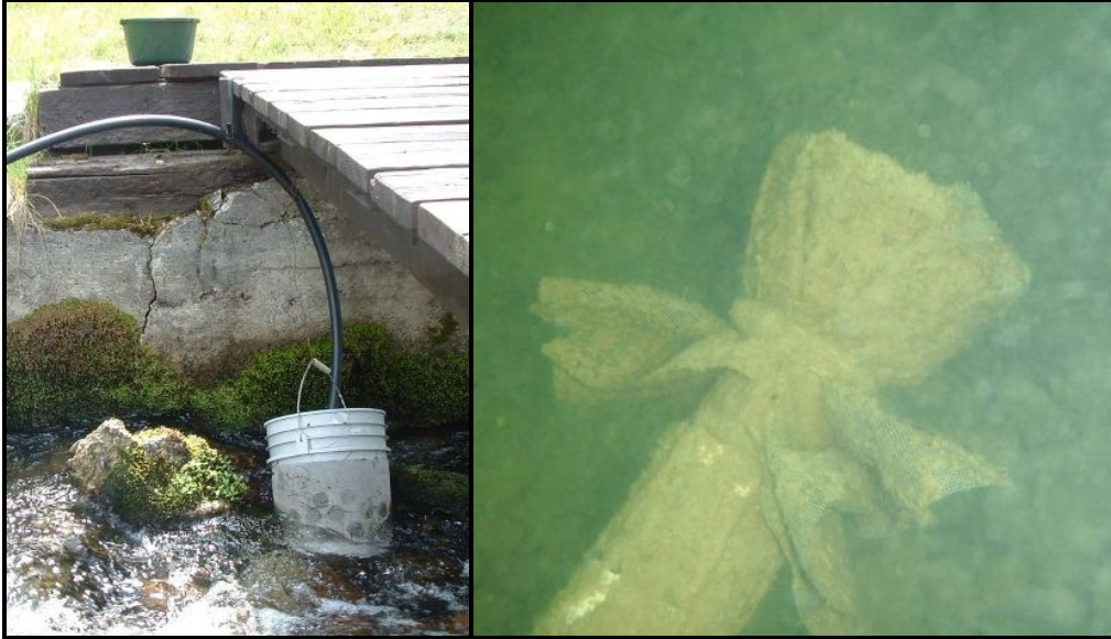
Figure 9.4. Informal or homemade screens. Informal diversion screens are not considered adequate for the protection of fish life, and inventory crews should not indicate that a screen is present.
