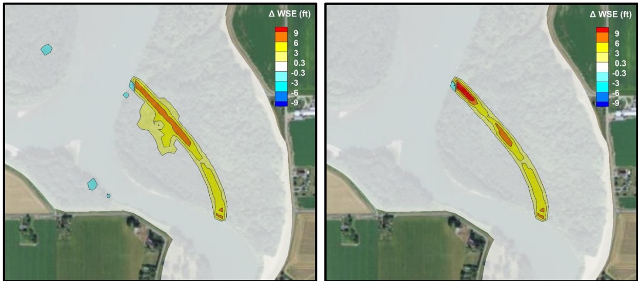
Figure B.44. Contour map of change in WSE from the Baseline to Small Projects simulation for East Cottonwood with Q2 flow and low tide (left) and flood flow and high tide (right).
