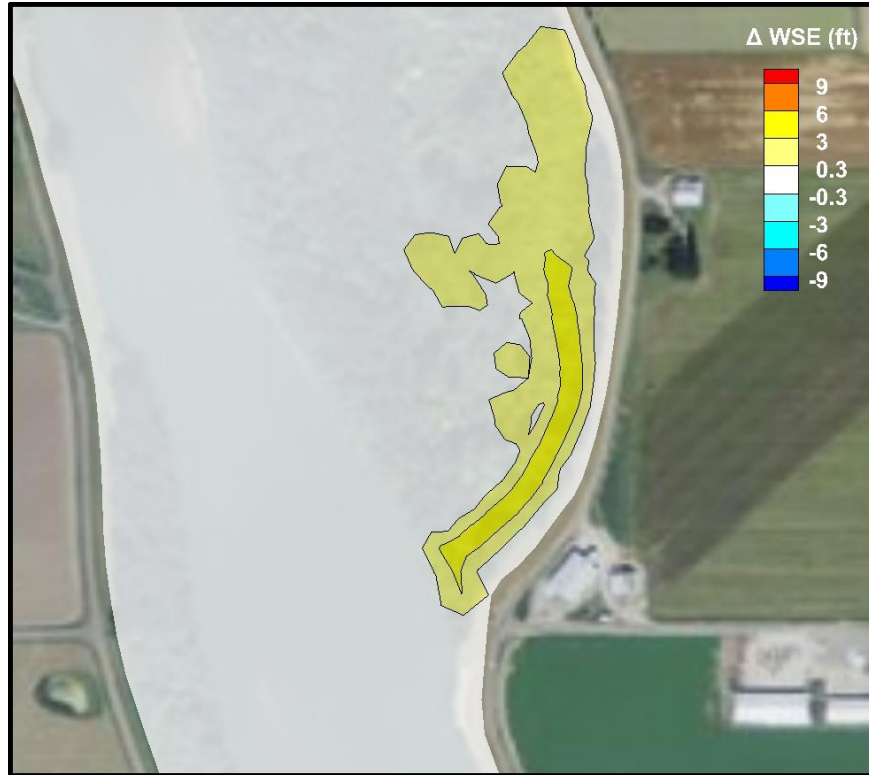
Figure K.45. Contour map of change in WSE for low flow and high tide for TNC South Fork, comparing Climate Change Baseline and Climate Change Projects simulations.
