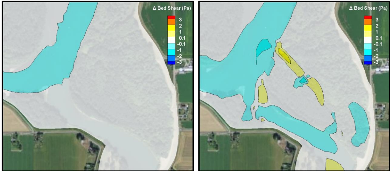
Figure B.57. Contour map of change in shear stress from the Baseline to Small Projects simulation for East Cottonwood with peak shear across a full tidal cycle at low flow (left) and Q2 flow and low tide (right).
