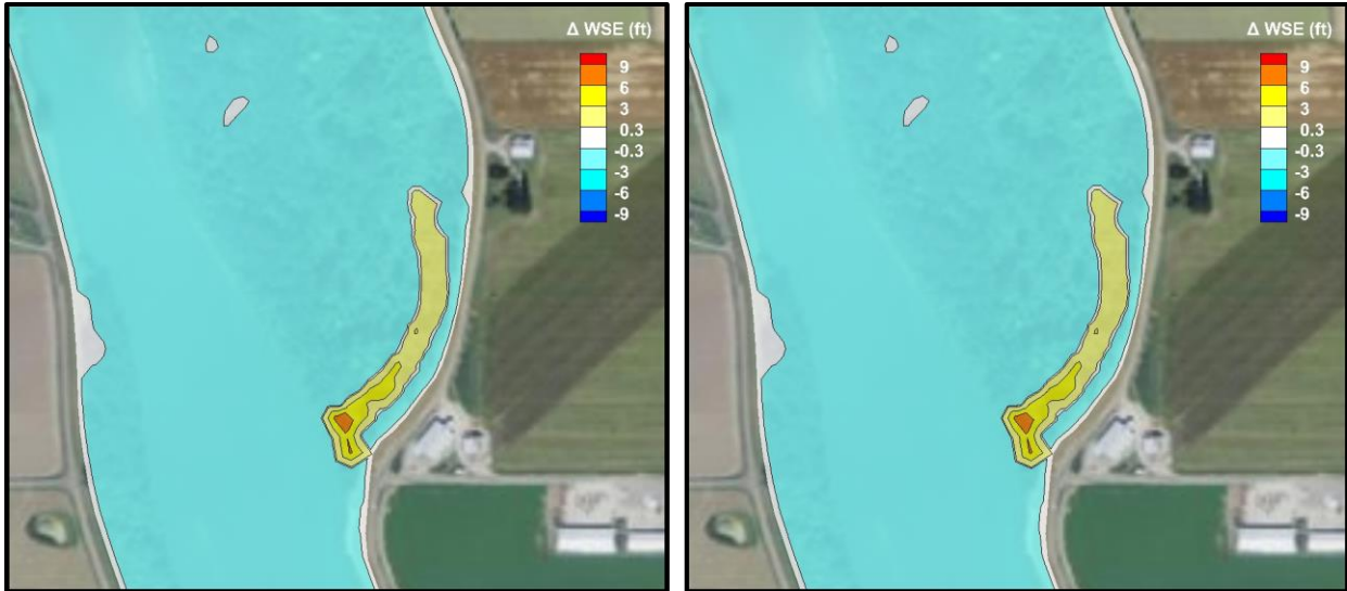
Figure K.6. Contour maps showing the change in WSE for TNC South Fork with a future Q2 flow and future low tide (left) and a future Q2 flow and future high tide (right), comparing Climate Change Baseline and Climate Change Projects simulations.
