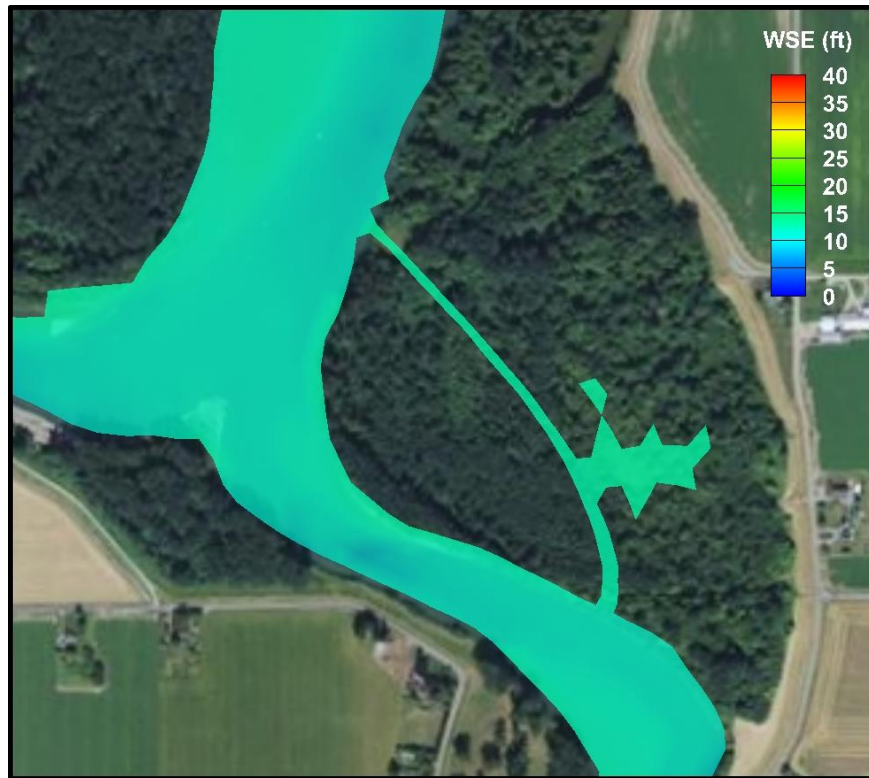
Figure K.66. Contour map of water surface elevation for East Cottonwood during the 2080 Climate Change with Projects simulation with low flow and future high spring tide.
