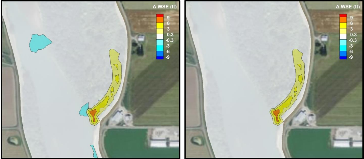
Figure B.42. Contour map of change in WSE from the Baseline to Small Projects simulation for TNC South Fork with Q2 flow and low tide (left) and flood flow and high tide (right).
