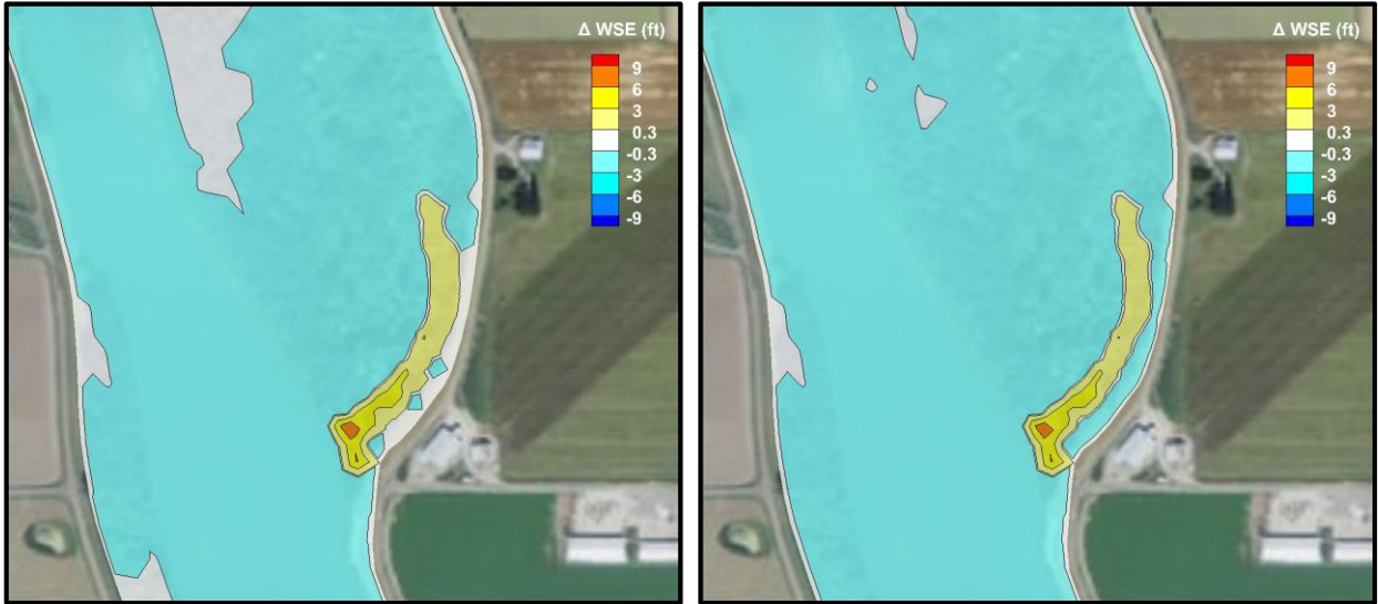
Figure I.52. Contour map of change in WSE from the Baseline simulation for TNC South Fork with Q2 flow and low tide (left) and flood flow and high tide (right).
