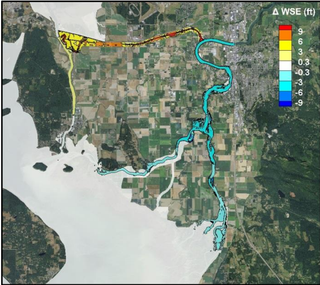
Figure D.9. Contour map of change in WSE from the Baseline to Avon-Swinomish Bypass simulation with flood flow and high tide.
