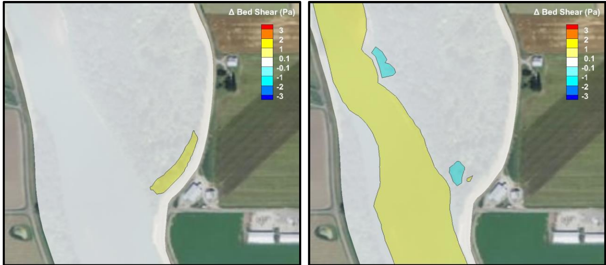
Figure B.55. Contour map of change in shear stress from the Baseline to Small Projects simulation for TNC South Fork with peak shear across a full tidal cycle at low flow (left) and Q2 flow and low tide (right).
