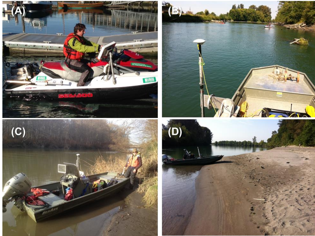
Figure 5. Photographs of the sonar data collection platforms including personal watercraft (A), small skiffs (B, C) and topographic surveys (D).
