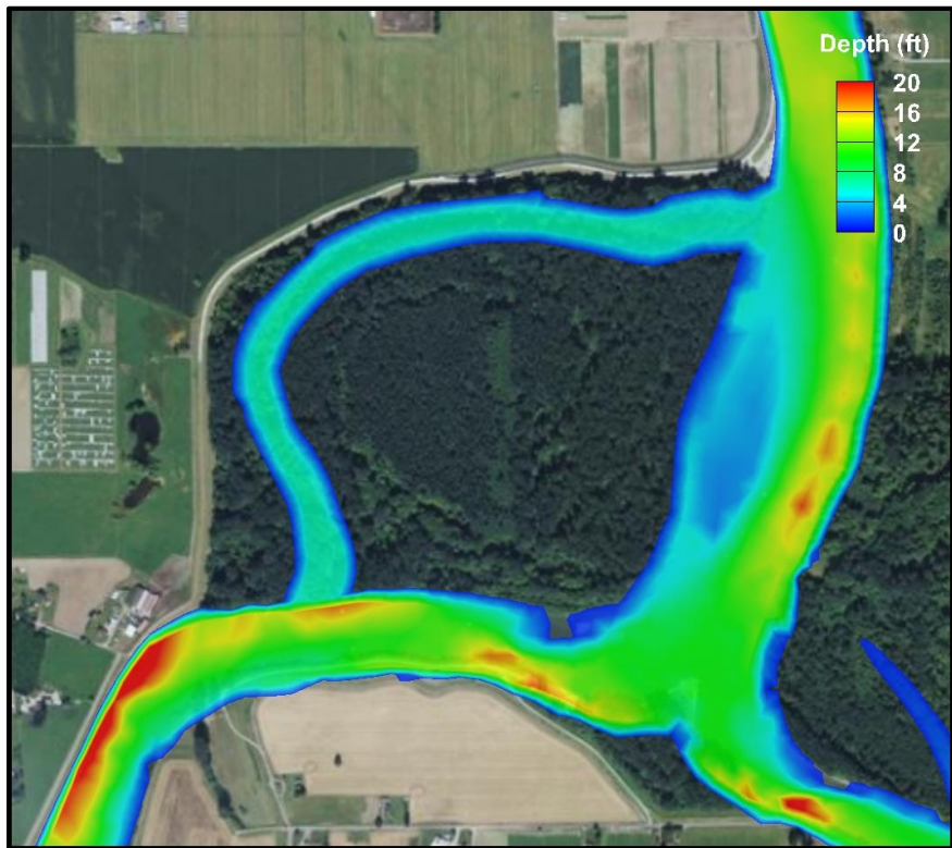
Figure I.33. Contour map of depths for Cottonwood Island during the Selected Projects simulation.
