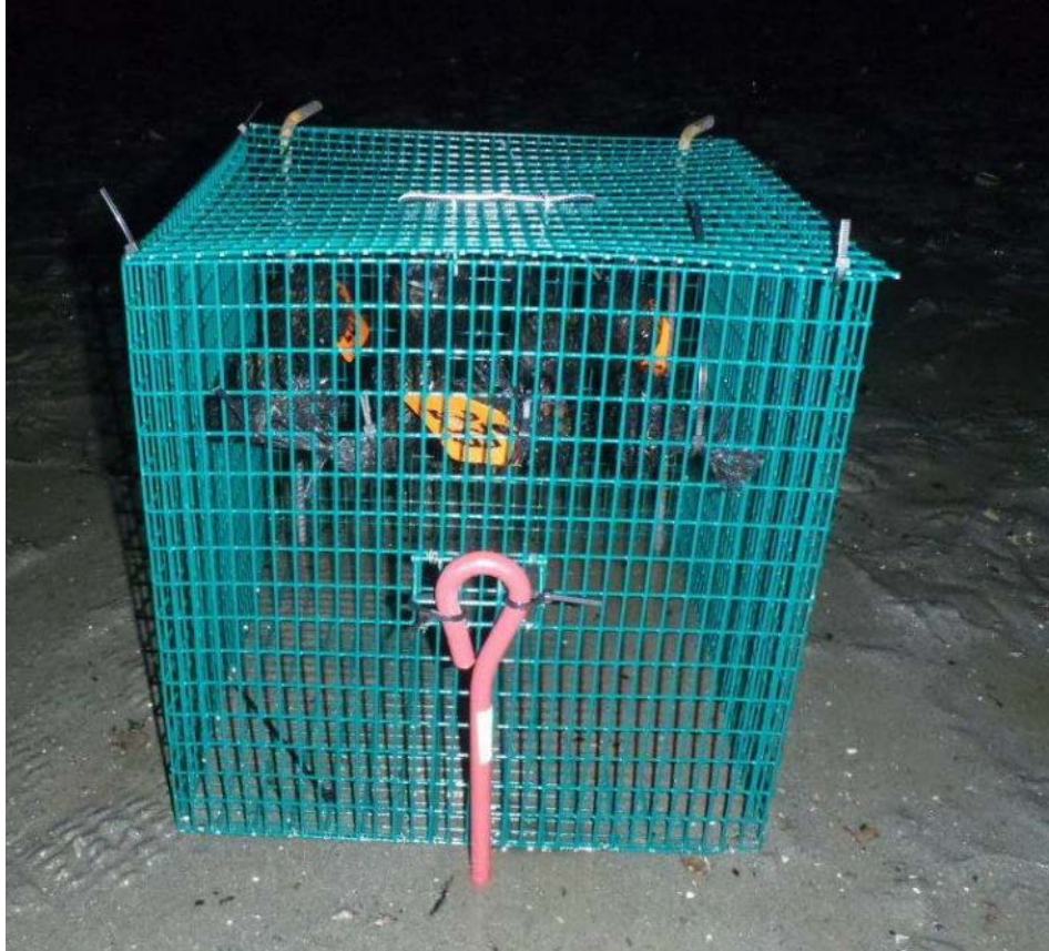
Figure 10. Mussel monitoring cage driven through with bent-tip rebar stakes (on the far end) and secured to a helical anchor with cable ties. For better cage anchoring, 3-4 rebar stakes are recommended.
