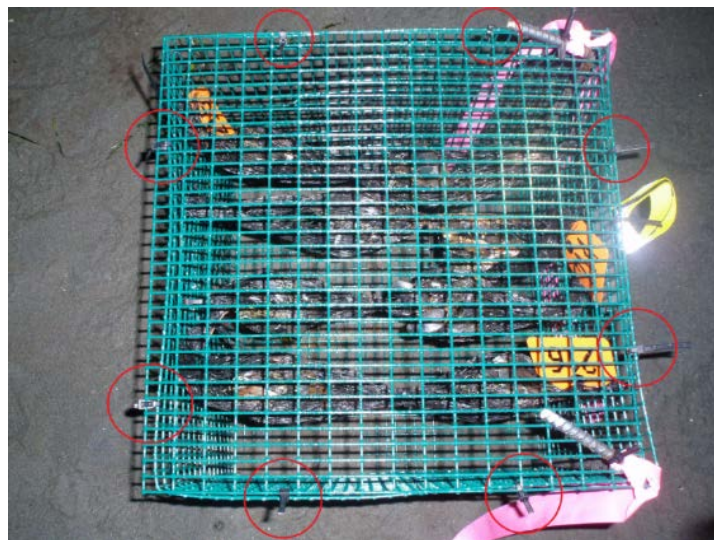
Figure 8. Anti-predator cage lid secured in place with at least two 8-inch cable ties per edge (red circles).
