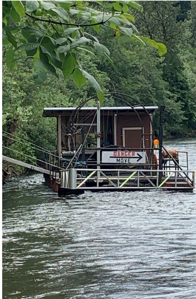
Figure 2. Chehalis River screw trap under low flow fishing conditions.
